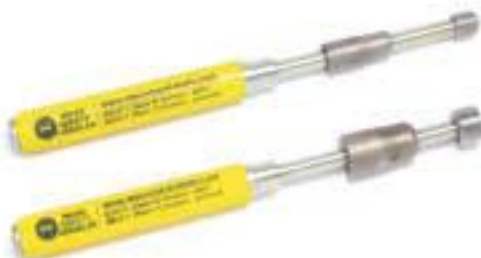
Patented tool for removing 15mm, 22mm and 3/4" olives. Engages with 14tpi thread of the compression fitting.
