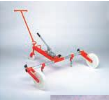
Hydraulic manhole cover lifter is quick to assemble and simple to use. The lifter can give up to 1.5 tons of lift, making easy work of the heaviest manhole cover. The lifter is supplied with 4 sets of keys which will enable most types of cover to be lifted. Weight 25kg.
