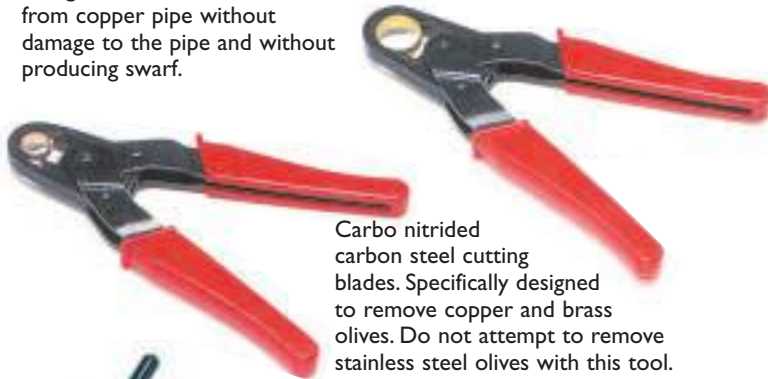
Patented tool for removing 15mm, 22mm and 3/4" olives. Engages with 14tpi thread of the compression fitting.
