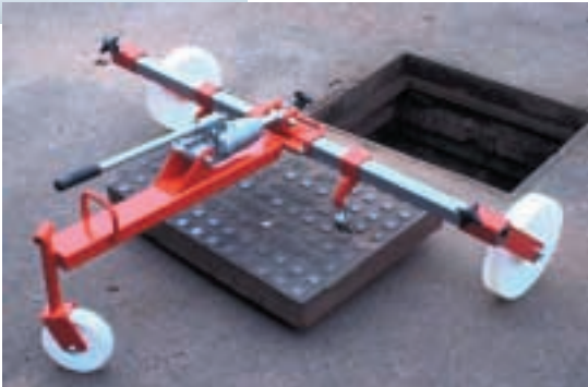
Hydraulic manhole cover lifter is quick to assemble and simple to use. The lifter can give up to 1.5 tons of lift, making easy work of the heaviest manhole cover. The lifter is supplied with 4 sets of keys which will enable most types of cover to be lifted. Weight 25kg.
