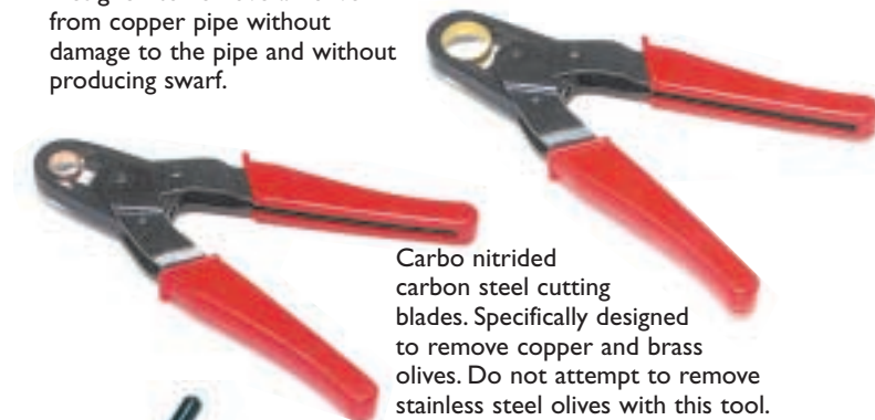
Patented tool for removing 15mm, 22mm and 3/4" olives. Engages with 14tpi thread of the compression fitting.
