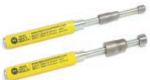
Patented tool for removing 15mm, 22mm and 3/4" olives. Engages with 14tpi thread of the compression fitting.
